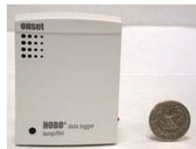
Figure 3. HoBo relative humidity and temperature logger.
