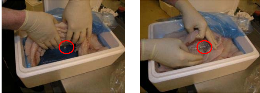
Figure 12. Left: Temperature logger placed at the bottom of an EPS box. Right: Temperature logger placed in the middle of an EPS box.
