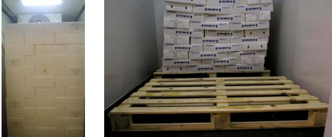
Figure 8. Left: Whole pallet with EPS boxes. Right: Pallet with Coolseal boxes not showing the two uppermost rows. The pallet in front of the Coolseal pallet was loaded with EPS boxes.
